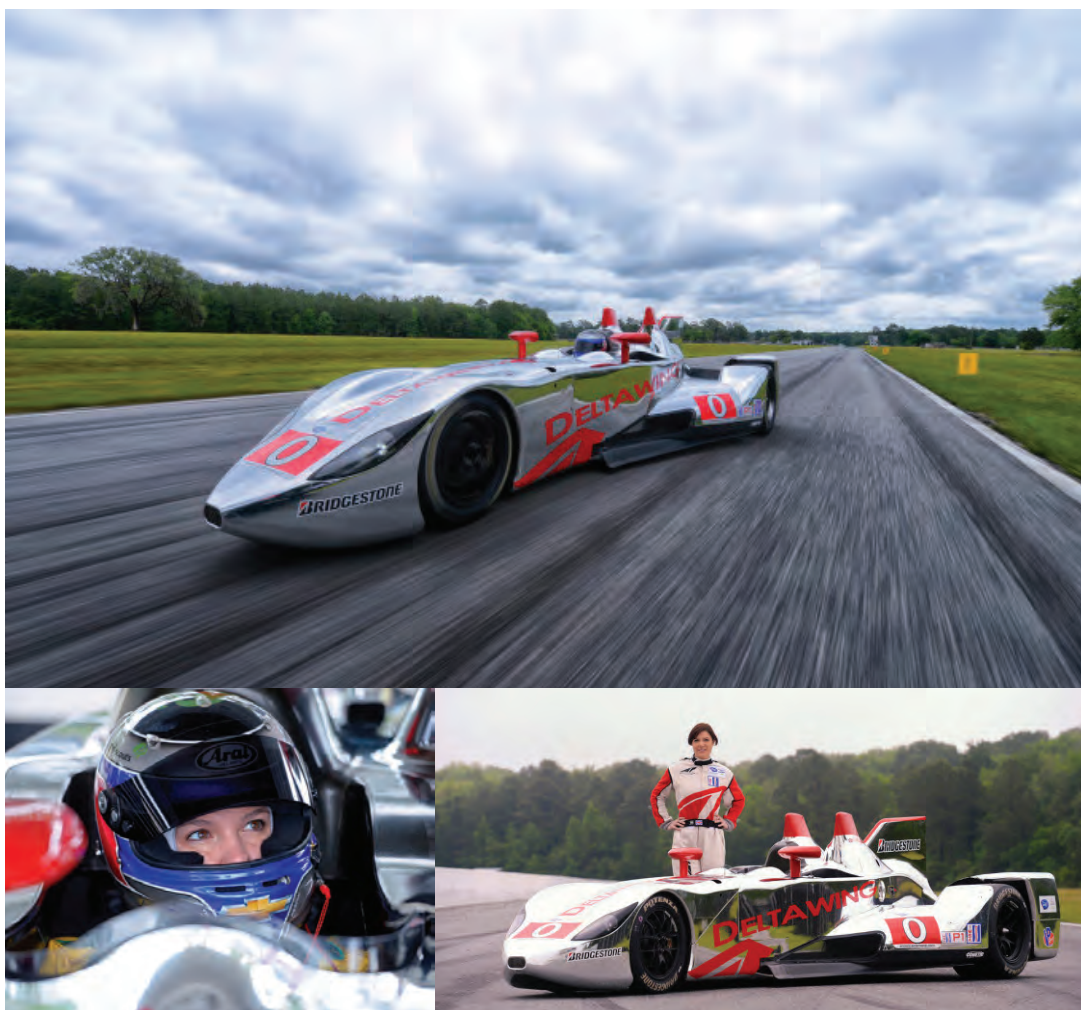
Above: Katherine Legge with the DeltaWing which “embodies a new era of eco-friendly technological advancement, with nearly half the weight, aerodynamic drag, horsepower and fuel consumption of its competitors.” Photos courtesy of Katherine Legge’s website, www.katherinelegge.com .
